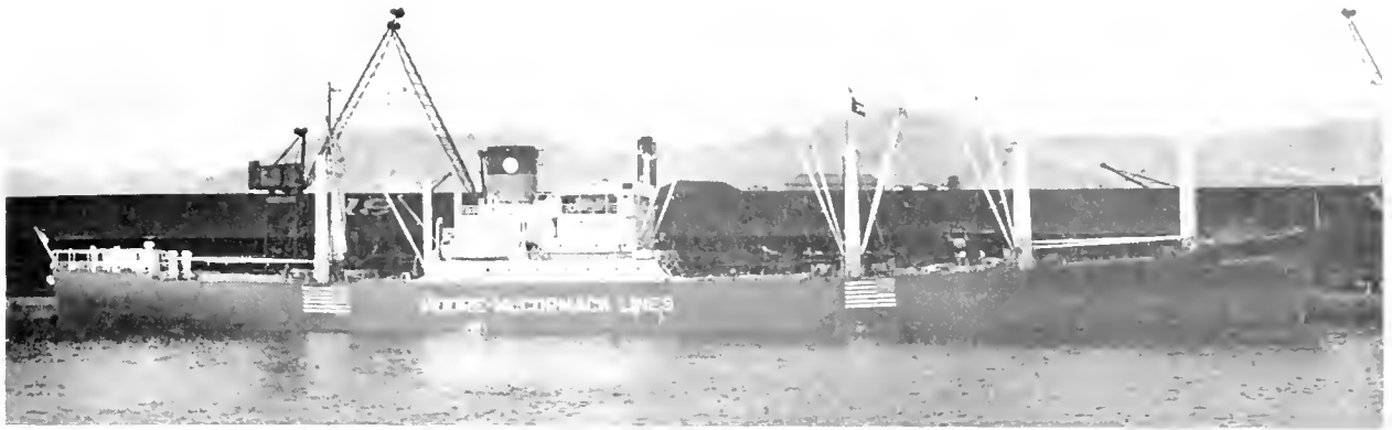
AMERICAN MERCHANT SHIP, CLASS C-2, MODIFIED FOR USE OF A PRIVATE OPERATOR. Many of this design were employed in war service. Rigger model USNM 313024 shows the basic design of the class. (U.S. Maritime Administration photo 1416.)
